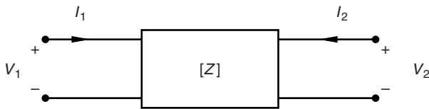
FIGURE 7.1 Two-port circuit expressed in impedance parameters.
